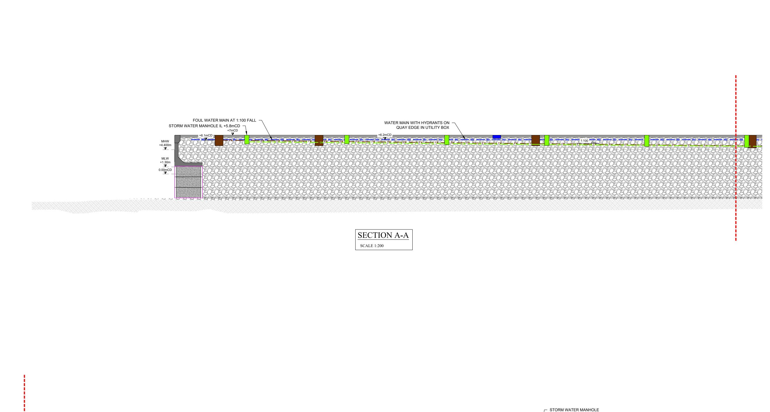
INLET IL +4.2mCD OUTLET IL+4.1mCD WATER MAIN WITH HYDRANTS ON -FOUL WATER MAIN AT 1:100 FALL -FOUL PUMPING STATION -/ SILT TRAP IL +4.0mCD QUAY EDGE IN UTILITY BOX ─ OIL INTERCEPTOR IL +3.9mCD 7mCD \_\_\_**▼**\_ OUTFALL IL+3.6mCD 2.2mCD -\_\_\_\_**▼**\_
